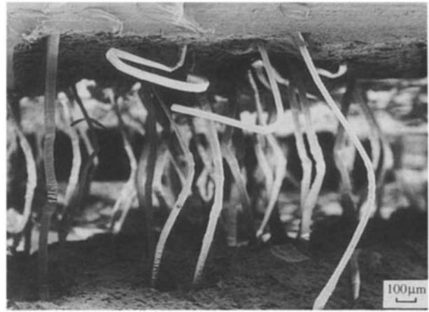
Figure 2 Surface topography of a fractured three-point bend loading test specimen reinforced with UHSPE-1000 virgin fibres of 6.35 mm lengths at 1 wt % fraction.
