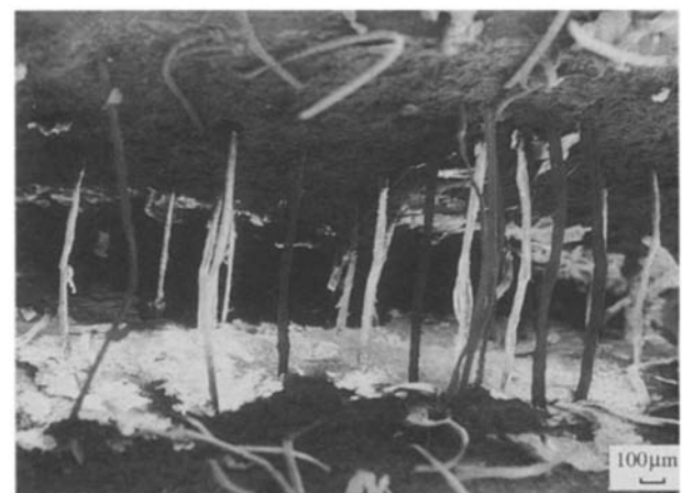
Figure 4 Surface topography of a fractured three-point bend loading test specimen reinforced with argon plasma-treated UHSPE-900 fibres of 6.35 mm lengths at 1 wt % fraction.
